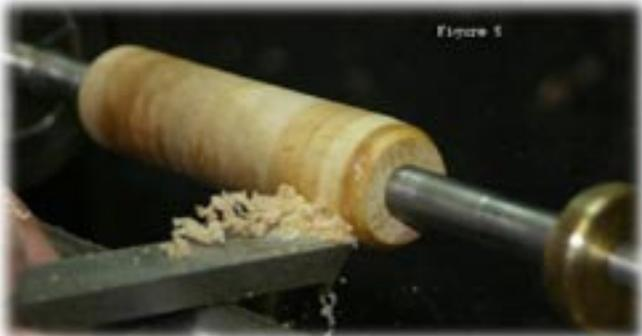
**Figure 6:** Applying the boiled linseed oil...3 drops...too much oil can lead to failure...A common cause of failure, blotches, ghosting, and globing. The amount of oil may need to be adjusted for your shop conditions. Three drops is not an absolute, but works for me.
