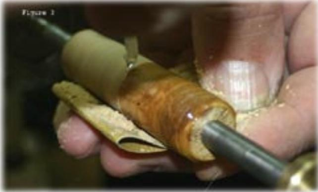
**Figure 4:** The blank as it looks after CA slurry and prior to removal excess slurry.
