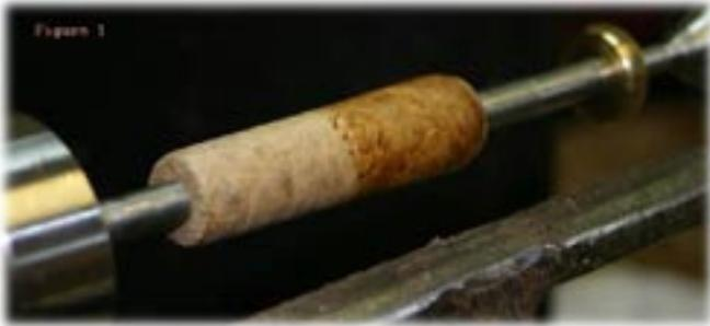
**Figure 2:** Collecting sanding dust with 180 grit to use for the CA slurry as a sealer. This step could be omitted and a sanding sealer used. The slurry works exceptionally well for open grain woods.
