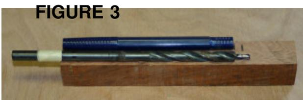
My next step was to lay the Foray body and the step bit for the Pentel on the chosen blank and mark lengths. I marked the end of the barrel and almost to the end of the drill bit. I put a piece of tape on the drill bit to indicate where to stop the drilling. I drilled then cut the blank to length.
