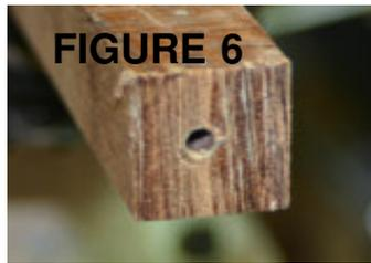
The end of the blank was cut off on the band saw. Notice the small hole made by the step .5/32 inch. But for the Foray pencil we need a larger hole. I use a letter B bit (.2308") Another size may work but the B bit is a close fit.
