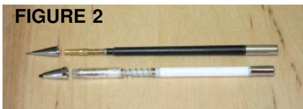
This photo shows the Pentel and the Foray mechanisms side by side. The Pentel tip is all metal. The Foray tip is all metal except for the black tip which holds the lead and is plastic. Note the end of the Foray mechanism is larger than the Pentel's. This is the problem I had to solve.
