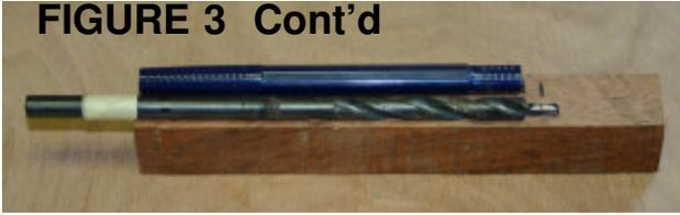
Notice the blank will be longer than needed but I have found it easier to cut it longer and shorten it on the disk sander and sneak up on the final lengths. I drill next and do the drilling on the lathe.
