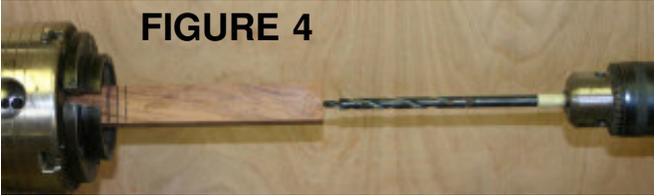
The blank is mounted in my chuck and the bit is aligned prior to tightening the chuck. Drilling can be done on a dill press but I find the lathe to be better for this.
