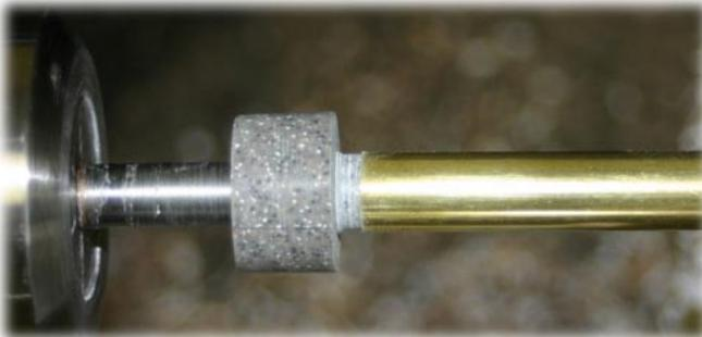
I then removed one of the partially made bushings and placed the sierra tube over the slimline bushings. I used sandpaper to get the final size of the bushing to insert inside the tube. The tube is used to find the correct size.
