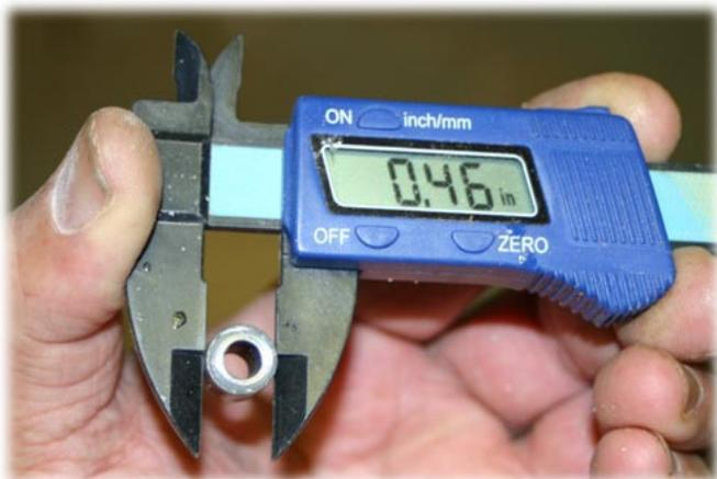
Measure the other end of the bushing. This end is the pen diameter end.
