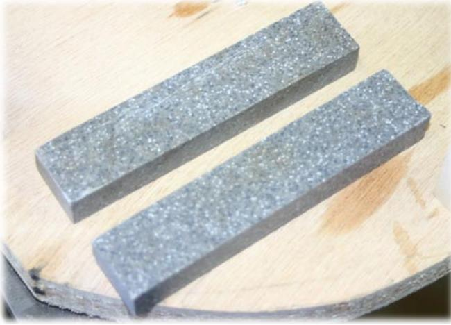
I choose to use corian for this tutorial. Aluminum could be used, but not hardware store stock. I use 6061 aluminum rod. This piece of corian is 1" x .5" and when glued together will be 1" square. I glued with CA.
