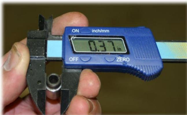
Measure the real bushing for future reference. This is the end that will go inside the brass tube from the pen kit. I've chosen to make sierra bushings for this tutorial.
